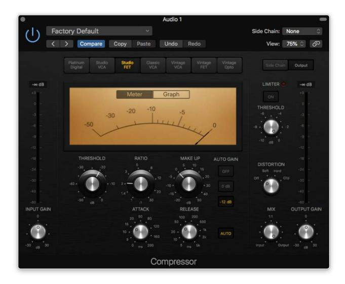
FET compressors are fast and punchy. Try this on drums. On the snare, on the kick, or even the drum bass. It was made for it!
