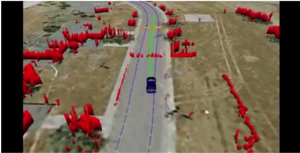
The only way for the car to navigate is to take multiple U-turns, and it had to plan it all by itself using A\* planning. The car pulls up to the barrier, realizes there is no valid path, and invokes its A\* planner to come up with a turnaround maneuver that is not particularly elegant, but is super effective. The car was able to turn around by itself using A\*, find the optimal plan to do so and then move on. Otherwise, it would have been stuck forever behind the obstacle.
