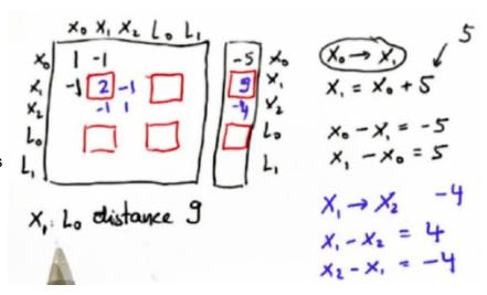
in the matrix and vector to indicate that landmark's  $L_0$  position is 9 greater than  $x_1$ .
