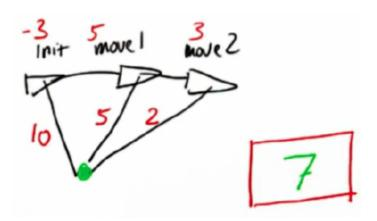
The equations used to reach this conclusion are shown in the table below. They are the same as the equations encoded in Omega and Xi. If you assume a fixed coordinate  $x_1$  for the landmark, the only value that works for all equations below is  $x_1 = 7$ .
