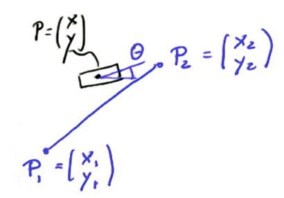
$x-x_1$  and Ry = y - y<sub>1</sub>. Then u, which measures the robot's progress along this segment, is given by the dot product:
