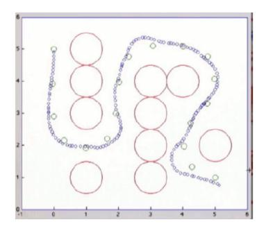
through a loop, where cross-track error, CTE is computed, then applies the PD controller (no I term there), and finally runs the particle filter, as before, to estimate where the robot is.
