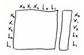
**1.** The equation is changed so that both x terms are grouped together and the term corresponding to the source pose, has positive sign:  $x_0 - x_1 = -5$ . Then, +1 and -1 coefficients for  $x_0$  and  $x_1$  respectively are added to the matrix which initially contains all zeros. The -5 constraint is added to the corresponding element in the vector.
