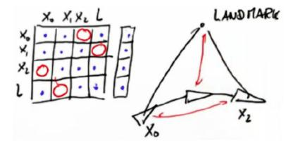
What this means is that there is no direct constraint between  $x_0$  and  $x_2$ , since there is no direct motion information between them, as well as no direct constraint between  $x_1$  and L, since there is no measurement information between  $x_1$  and L.
