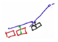
In addition to calculating the assigned error relative to an arbitrary line segment, not just the y-axis, you also have to detect when the robot steps beyond the end of a line segment and switch over to the next one.
