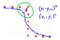
Although this new path suffers greater error from the  $||x_i - y_i||^2$  term, it drastically reduces the distance between points and therefore reduces the error from  $||y_i - y_{i+1}||^2$ , thus minimizing the overall function  $c_1||x_i - y_i||^2 + c_2||y_i - y_{i+1}||^2$ .
