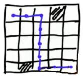
A path like this has many disadvantages. You don't want the robot to go straight, take a 90-degree turn, then go straight again. A car cannot even make a 90-degree turn, and this route will force the robot to move really slowly around the corners. A much better path would look like the red curve in this next picture:
