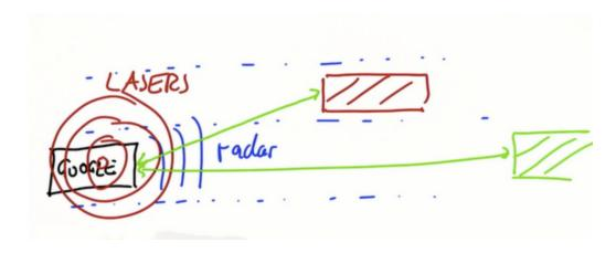
So, when the Google car is on the road it uses radars and lasers to estimate the distance and the velocity of other vehicles on the road using a Kalman filter, where it feeds in range data from the laser and uses state spaces of the relative distance, *x* and *y*, and the relative velocity of *x* and *y*.
